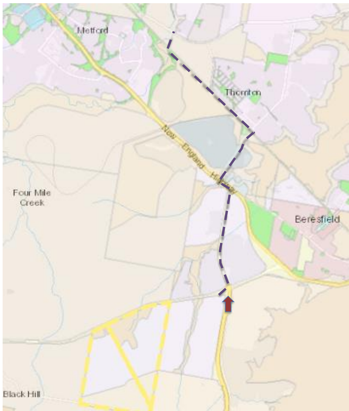
Figure 4: Proposed sewer shown in purple dashed line. Intersection upgrade in red arrow (ePlanning Spatial Viewer 2020).
