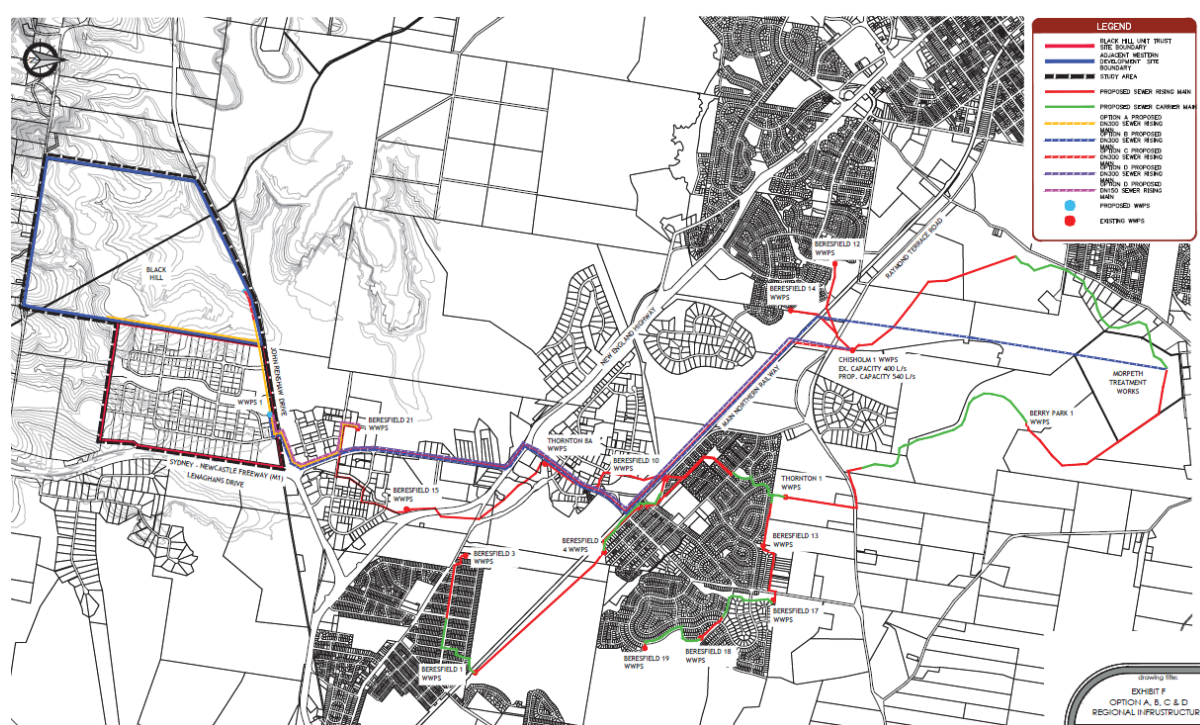
Figure 2: Sewer extension shown in purple (ADW Johnson 2020).
